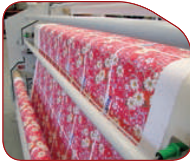
Even temperature and fabric-tensioning system Paper re-using system capable of feeding the fabric duly centered.
